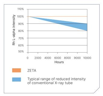
With Revontium, you can account for every signal in your XRF spectrum – thanks to careful design and high-quality hardware and software components. Revontium's close-coupling, patented X-ray tube was designed specially for the instrument, and its zero-evaporation technology advancement (ZETA) means it has very low drift. Together with features that protect against spillage, this enables long-term stability.
